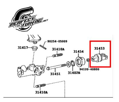
The extended cutter pin goes replace the factory one
